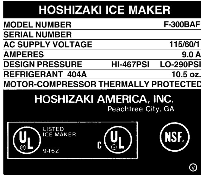
See the nameplate for electrical and refrigeration specifications. This nameplate is located on the upper right hand side of rear panel.
